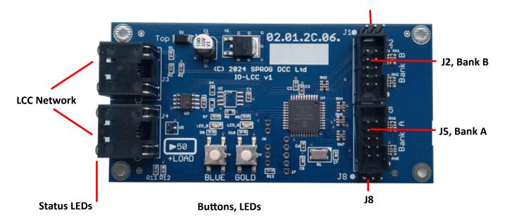
Three status LEDs are built in to the network connectors to indicate LCC power, message send and message receive. The LCC send and receive LEDs blink briefly for each message.
