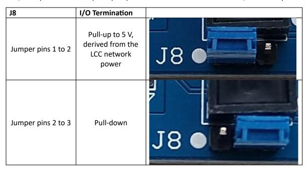
J8 Pin is denoted by the white circle on the top side of the PCB and the square pad on the bottom side.
