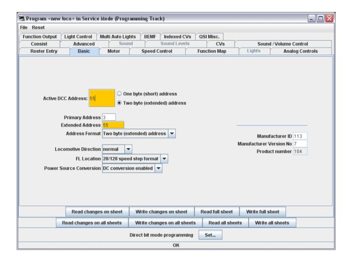
Click "Write changes on sheet" to write the new address to the decoder. The address will turn red and then white as it is written to the decoder. You can set other basic properties such as the direction and DC operation on this tab.
