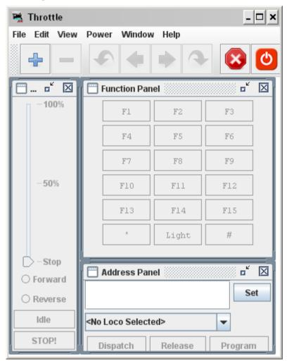
The Power icon on the right of the menu bar is the track power control and must be clicked until it is green to turn on the track power. The SPROG II power LED will flash when the track power is live.
