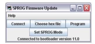
First the old firmware will be erased, and then the new firmware will be written. Progress is reported in the status line of the window. If the Console is still open, you will also see the messages flowing between the computer and the SPROG.
