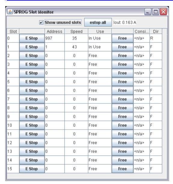
In this example, SPROG II is supplying 163mA to the layout. A loco with address 997 is running in reverse at speed step 35 and a loco with address 1 is running forwards at speed step 43
