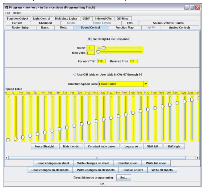
The decoder in this example has a choice between "Use Straight-Line response" and "Use QSI table or User table in CVs 67 through 94". The "look and feel" of this tab will vary between decoders but most recent decoders support the use of a speed table.
